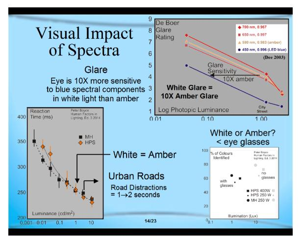
This slide compares three aspects of white and amber LED lighting. The top-right graph is from Dr. Derloske and Bullough (Rensselaer Inst.) at NHTSA Workshop. The luminance of the light with blue spectral components has to be 1/10 the luminance of amber light if it is to have the same glare impact. This demands better shielding, or reduced light output (1/10 wattage).
