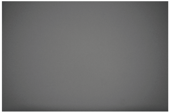
Figure 5 — Flat-field image. Note the effects of vignetting.
