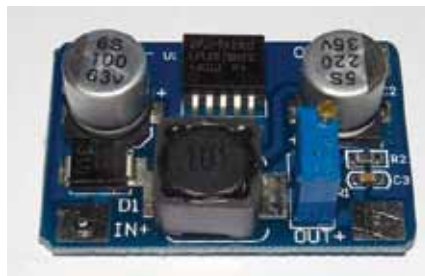
Figure 2 — The variable-voltage board.
