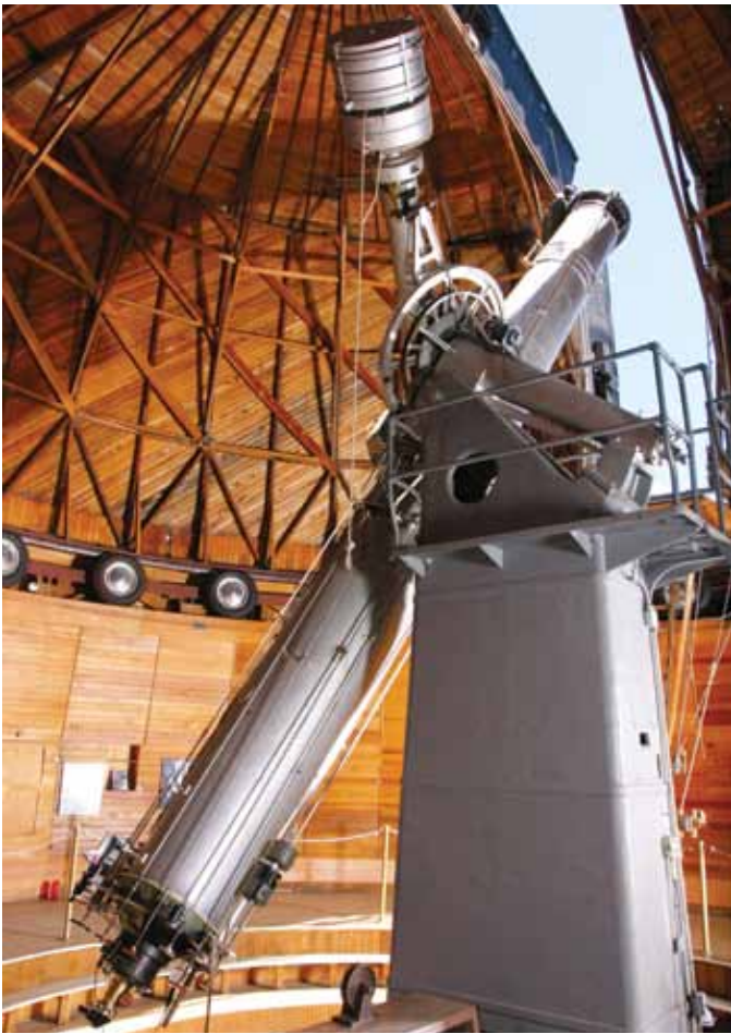
Figure 1 — The venerable 24-inch Clark refractor in its wooden dome. (Except where noted, all images courtesy Lowell Observatory)
