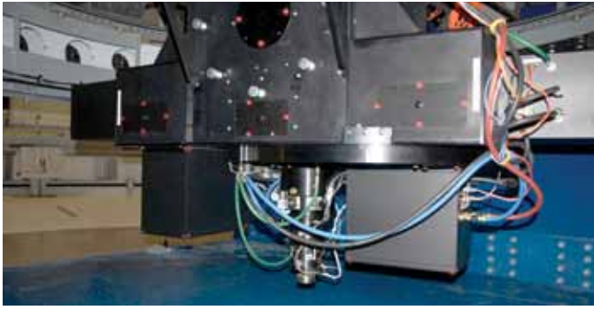
Figure 4 — The DCT's 2 \times 0.5 -metre instrument cube behind the primary mirror.
