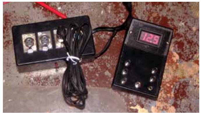
Figure 6 – The finished power-distribution box.
