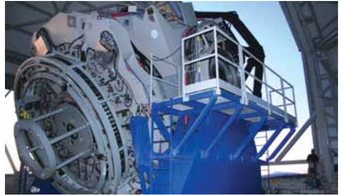
Figure 5 — Side view of the DCT inside its dome prior to installation of the instrument cube. Note the astronomer at right for scale. (Photo by M. Beckage)
