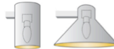
Compliant fixtures Good design
