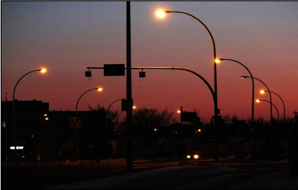
This evening photo well illustrates the lack of glare from full cut-off fixtures, such as the fixture third from the right. The glare of the cobra-head streetlights reduces the exposure of the camera, much as in the human eye, leaving the ground area darker and less visible while creating safety concerns.
