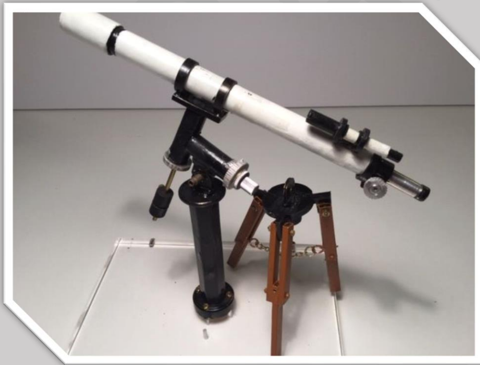
Unitron 5-inch O.G. f/15 refractor, with pier, and tripod.
