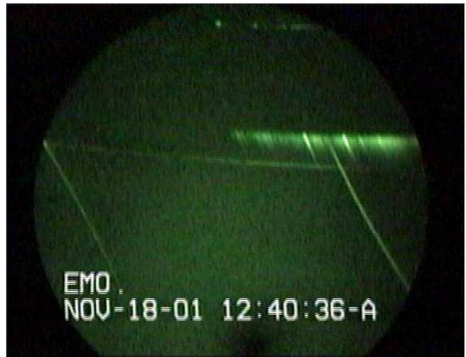
This spectrum was secured using simple equipment. An experimental grade type MX9944/UV 2nd generation 25 mm diameter image intensifier purchased on the surplus market was used.
