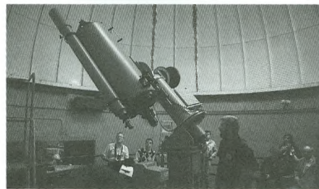
The workings of the 20" f/15 Cassegrain telescope at the Gordon Southam Observatory are being demonstrated by Dave Dodge (foreground). Photo by Patrick Kelly.
