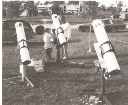
The three telescopes ( 1/2 , 1/4 , and 1/10 wave) from the Sky & Telescope optical quality experiment.
