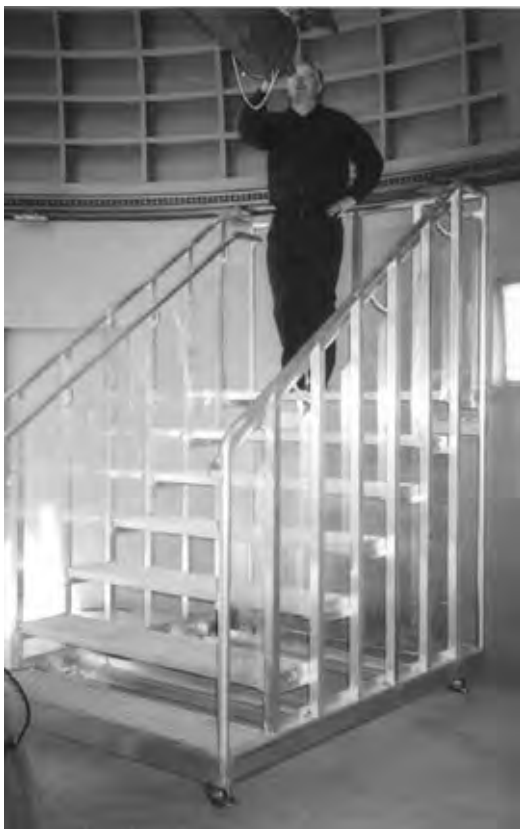
Figure 2 – The new observing platform designed and built for use in Jewett Observatory on the campus of Washington State University. The author Steve Mallory is seen standing atop the platform.
