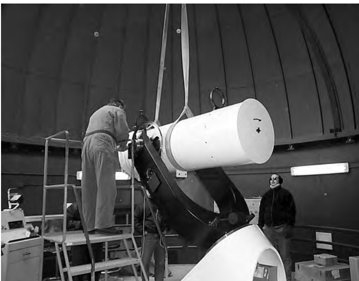
Figure 3. Pat Lavigne connecting the telescope tube assembly to the fork.
