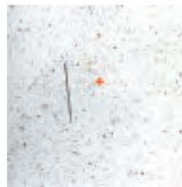
Figure 5 — An image of a Russian SL-3 rocket body (#13771) captured by my ST-9XE’s CCD camera while pointed at my local zenith at 23:48:45 UTC on February 11, 2006. The location of my local zenith at that time is denoted by the large red cross. The image field of view is about 11.2 \times 11.2 degrees. North is at top, east is at left. The exposure time was five seconds.
