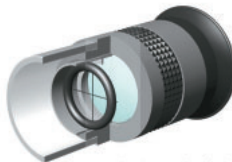
A cut away view showing the o-ring and cross hairs as they should be located inside the lens element retaining tube.
