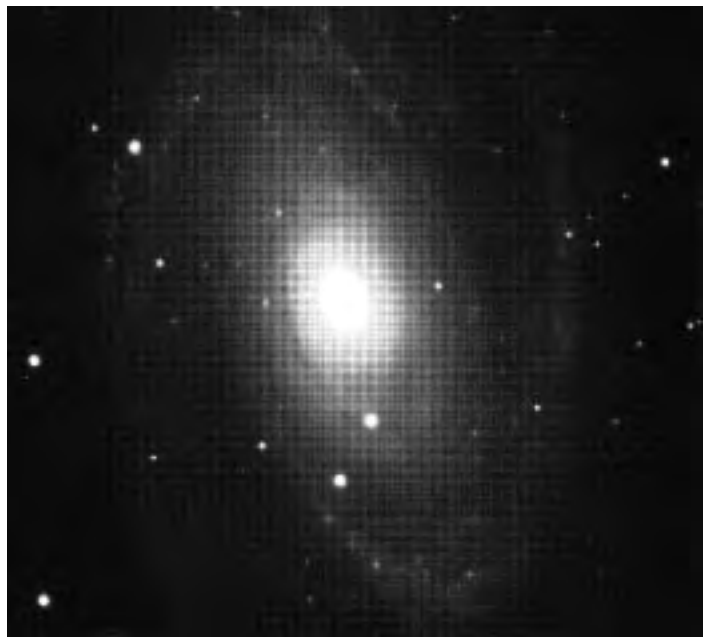
Figure 1 — Unprocessed image of M81 showing a Bayer matrix superimposed on the image.
