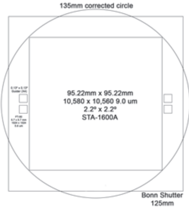
Figure 11 — The focal plane of the OMI camera showing the main sensor, guiders, corrected field, and shutter.
