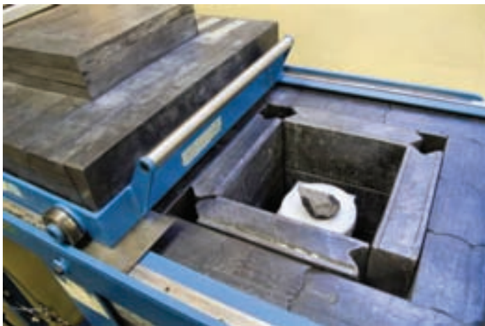
Figure 4 — The largest specimen recovered by Bruce and Frank was some 7 cm along its longest axis, just right to comfortably fit within this 15-cm “lead cave” at the SLOWPOKE nuclear reactor at the University of Alberta where its isotopes were counted for seven days. ©Department of Earth and Atmospheric Sciences, University of Alberta. Used with permission
