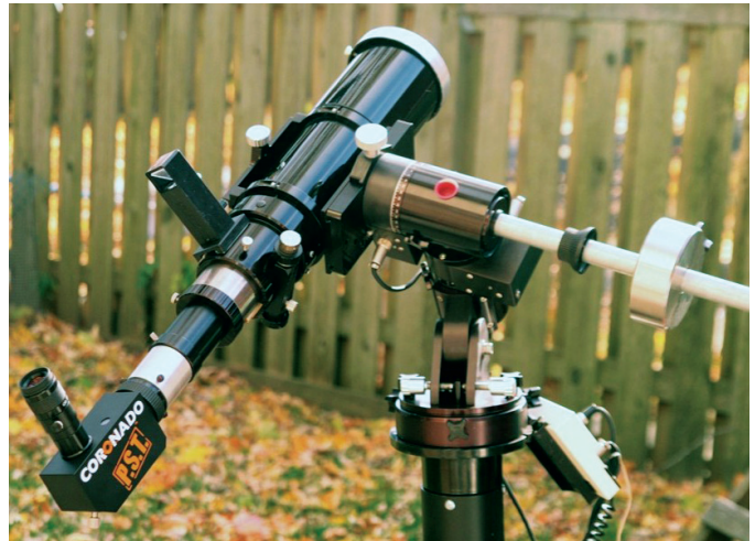
Figure 3 – An early 80-mm PST attempt using a 2× Siebert telecentric Barlow, AP f/6 Traveler, and Daystar 80-mm ERF.
