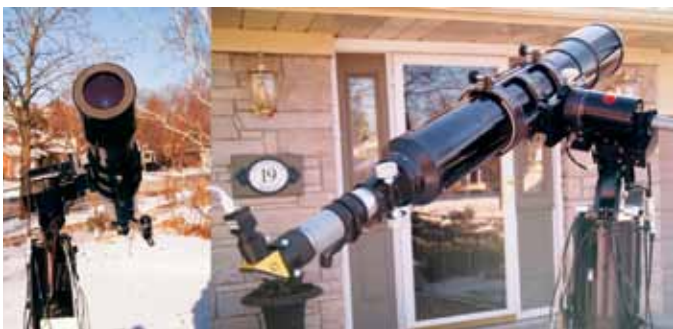
Figure 5 – 5-inch (127-mm) monster PST with 6-inch (152.4-mm) Celestron achromat and Rosco UV/IR blocking filter in a masked-down lens cover.
