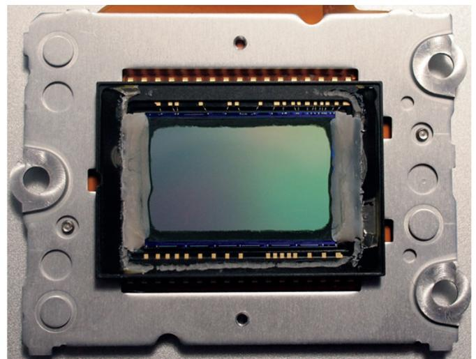
Figure 5 — Appearance of first successfully stripped D40 Sensor.
