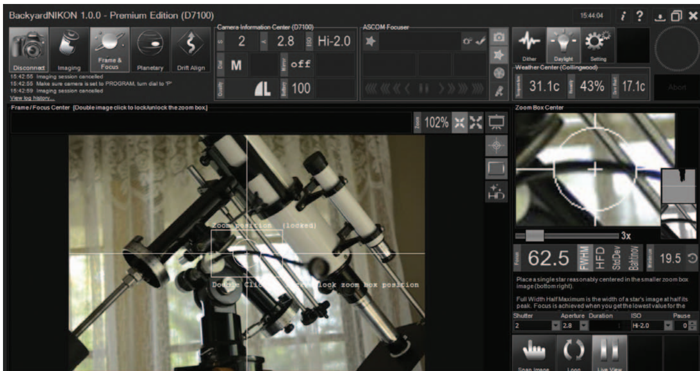
Figure 4 — When the Drift Align module is active, a reticle is displayed, superimposed over the Live View display. Submarine lighting, via the Daylight button, is clearly enabled.
