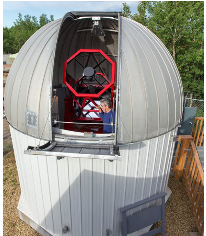
Figure 2 — The UDT seen from outside its dome the day after it was installed in July 2023. The 32" f/4 primary mirror can be seen at the base of the optical tube assembly.
