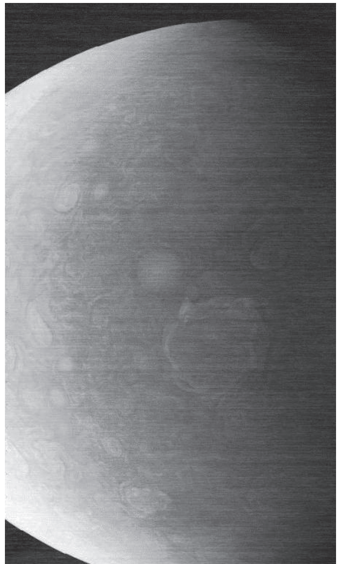
Figure 3 — The graininess and horizontal lines seen in this JunoCam image show evidence that the camera aboard NASA's Juno mission suffered radiation damage. The image was taken 2023 November 22. Credit: NASA/JPL-Caltech/SwRI/MSSS
