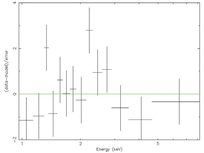
Figure 4 — The deviations from an absorbed power-law model (green line) for the Jan. 2018 epoch data. The model used is `tbabs*zpowerlw` in XSPEC and the data were grouped by a minimum of 10 counts per bin. The column density was fixed at  $N_{\text{H}} = 7.5 \times 10^{20}$  cm $^{-2}$  and the redshift at  $z = 0.0098$ . The data (crosses) show excess near 1.3 keV and 2.2 keV. See the Results section for more details.
