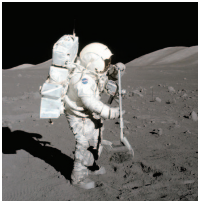
Figure 2 — Apollo 17 scientist-astronaut Harrison H. Schmitt collects lunar rake samples at the Taurus-Littrow landing site. This rake was used to collect samples ranging in size from 1.3 centimetres to 2.5 centimetres.
