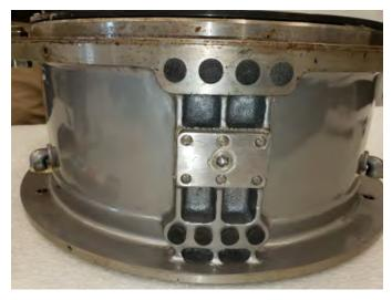
Figure 5 — Side view of the massive Perkin-Elmer lens cell. Photo by James Gort, courtesy of Canada's Museum of Science and Technology.
