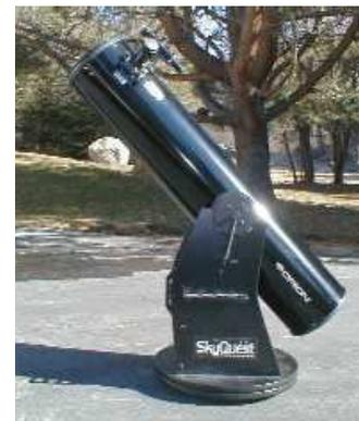
Reflectors use mirrors, coated on the front surface with aluminum, to collect and focus light. Better systems use Pyrex mirrors; cheaper telescopes have plate glass mirrors. In a Newtonian reflector light enters the tube, strikes the large primary
